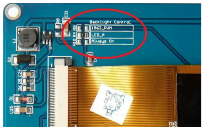
Simple driver to allow SPI ILI9341 LED-A pin to be driven by Backlight command. 0(off) to 100(fully on). VCC is 3.3V (SPI ILI9341 has no built in driver)
